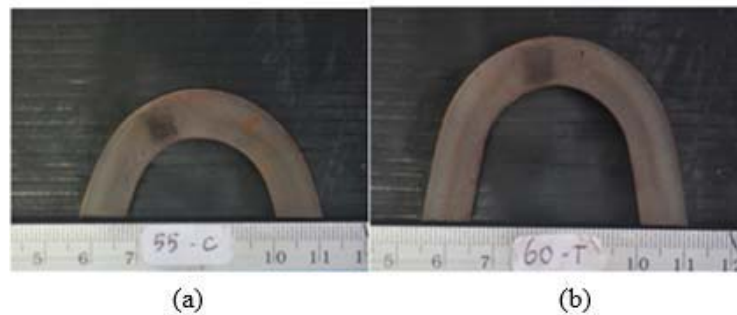
Figure 3. Material bending radius (a) 55 mm and (b) 60 mm
