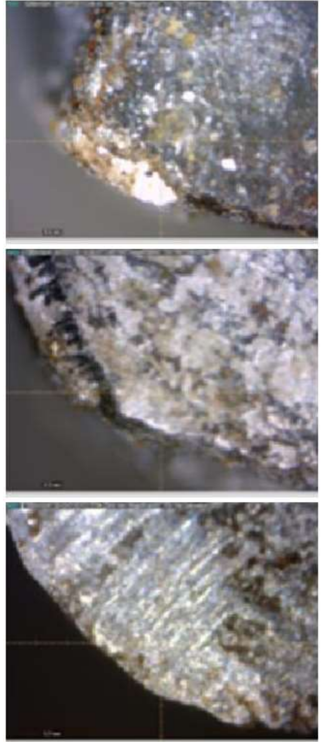
Figure 7: Optical micrographs at rake surface of ADI cutting tool with nitrogen cooling treatment, soaking 24 hours, continued by turning process V_c : 70 mm/min, f : 0.1 mm/rotation, for Al T-6061 a. Cutting depth a: 0, 1 mm b. Cutting depth a: 0, 5 mm c. Cutting depth a: 1, 0 mm
