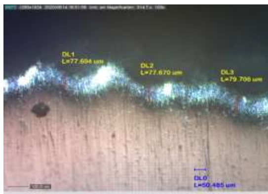
Figure 8. The oxide coating thickness resulted from the anodizing process with a 100% solution type 1M Sulfuric acid ( \text{HNO}_3 ) with a voltage variation of 15 Volt and immersion time of 30 minutes using a 100x optical microscope
