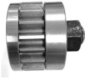
Fig 2. Fixturing the gears in the carburizing process
